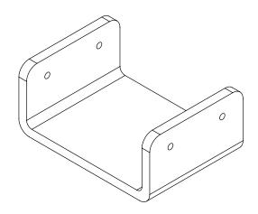
No adapter required if U saddle is welded to TMP
